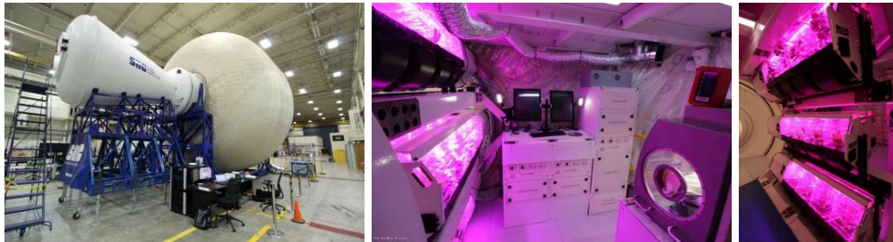
Figure 5. Sierra Space LIFE module mockup. Left-view of inflatable structure. Center and Right-Interior views of habitat.
