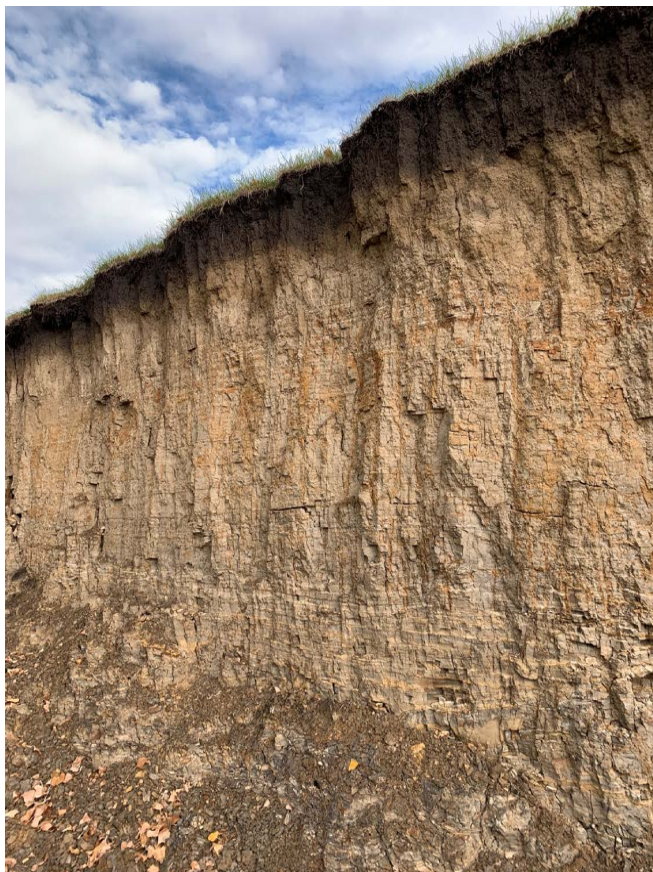
Figure 1. View of an exposed Overly? soil profile on the face of the slump
