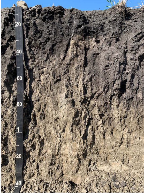
Figure 11. An Oxyaquic Hapludert on a lake plain dip formed in glaciolacustrine sediments
