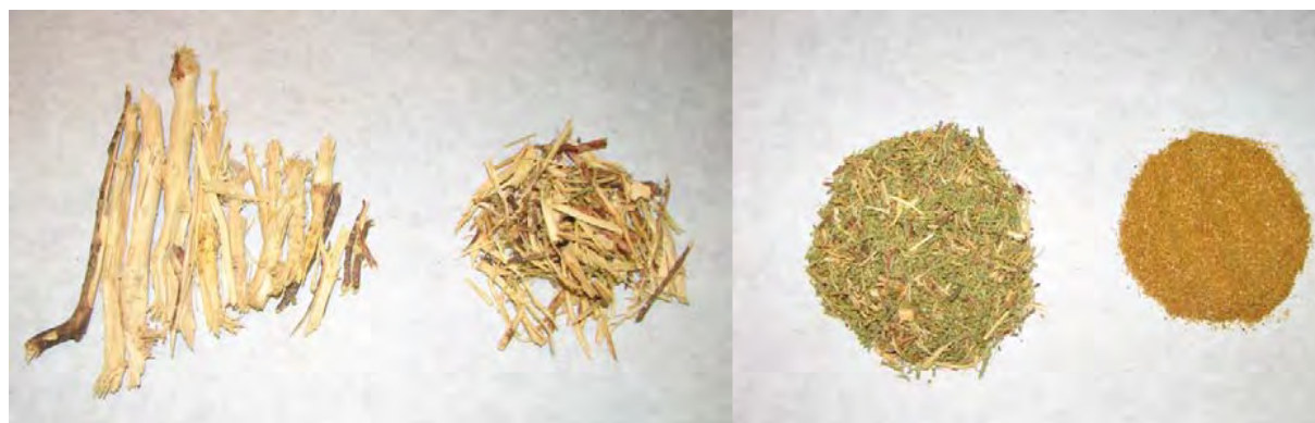
Fig. 1. Particle distribution of material separated by the Penn State particle separator. From left to right: material remaining on 19.0-, 8.0-, and 1.18-mm sieves, and in the bottom pan (<1.18 mm). Average particle length of material remaining on the top sieve (>19.0 mm) were measured manually and used as the geometric mean length because stem material on the top sieve was greater than 10 g/kg of total sample mass (ASAE #S424; 2007).
