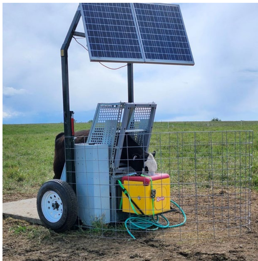
To determine daily grazing feed intake for individual heifers, researchers use various tools, including virtual fence collars (top) and a mobile heifer unit (bottom) that provides real-time measurements of body weight and water intake. Photos by Matthew Wilson, West Virginia University.
